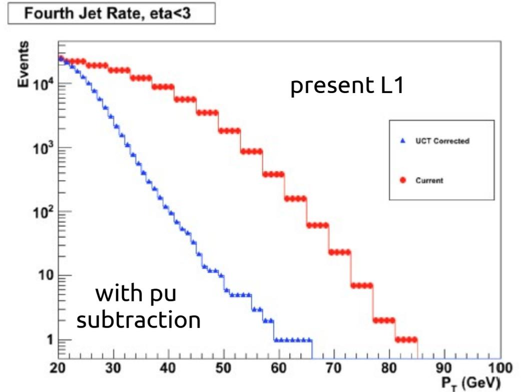
effect of pile-up subtraction on energy sums and multi-jet trigger
