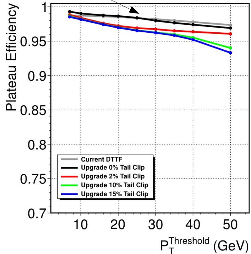
new muon  $p_T$  assignment (bigger LUTs, post-processing)
