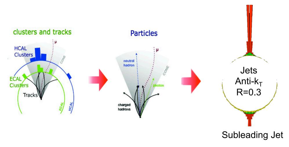
Calorimeter clusters and tracks are matched and combined to obtain most detailed information of particles in the event
